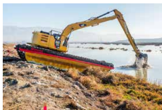
Amphibious excavator dipping its bucket into Pond A19 (©Julie Kitzenberger)
